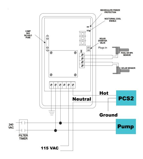
GL-235 with high voltage output used for SolarAttic PCS2
