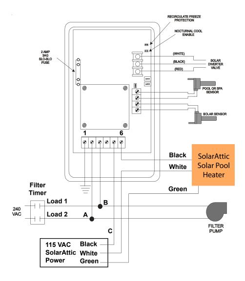
**POWER NOTE:** 115 vac is present at points A and B as measured to ground and if sufficient current is available, either may be used at point C to power the SolarAttic unit by connecting point A or B to C. Neutral and ground is routed directly to the SolarAttic outlet box in the attic. The hot side of 115 vac to the SolarAttic outlet box is supplied from terminal 6 (GL-235 relay output).
